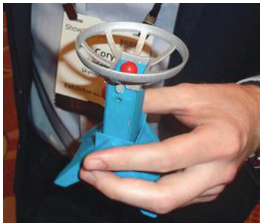
2. The pylons have an IR emitter allowing the drone to track its relative position.
