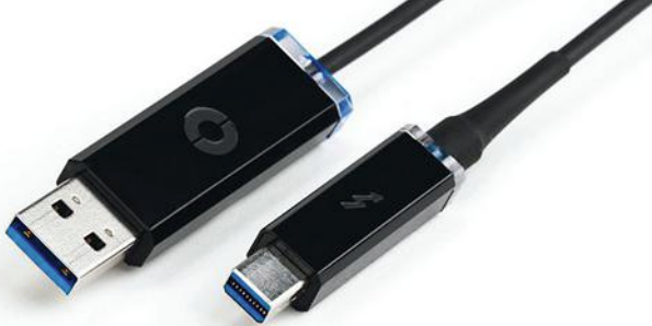
2. Corning's USB 3.0 uses standard USB connectors that incorporate transceivers at both ends. Two embedded fiber cables are used for data transmission, and a pair of copper connections provides power between transceivers.
