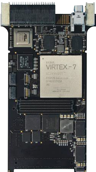
8. Pentek's Model 5973 Flexor Virtex-7 Processor and FMC Carrier board supports the optical VITA 66.4 standard.
