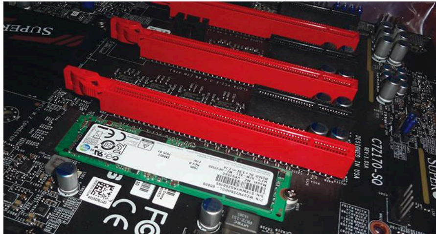
3. Samsung's 256-GB SM951 M.2 module is plugged into Super Microcomputer's C7Z170-SQ gaming motherboard.
