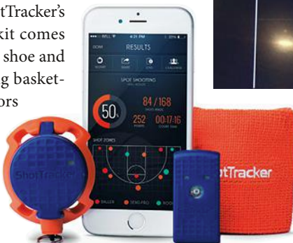
1. The ShotTracker starter kit includes a small tag on each player's shoe and the ShotTracker-enabled Spalding basketball connects with portable sensors placed around the court.
