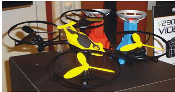
2. The pylons have an IR emitter allowing the drone to track its relative position.
